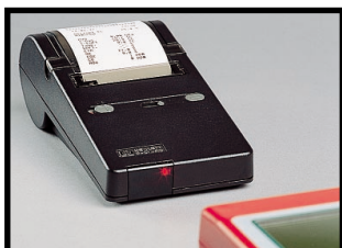
The well legible freely programmable print via infrared thermo printer contains all measuring data as well as the manually entered and stored soot spot number including the customer name and address, if necessary service print for easier error diagnosis, e. g. O 2 sensor failure.
