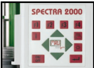
6 The new operator's guidance (via functional keys) is simple, serviceable and menu-guided with display-memory-function.
