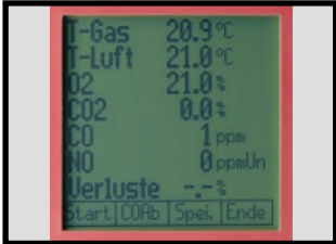
4 The very large display (6,5 cm x 6,5 cm) with 7 measured values at one glance is pleasant for your eyes and saves time-intensive scrolling of the display.
